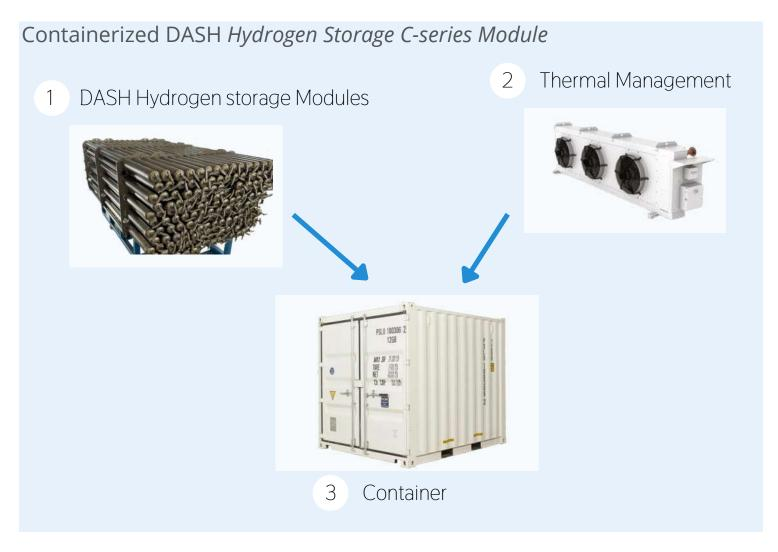
By creating a containerized modular design, we offer four different versions of the DASH C-series Hydrogen Storage Modules, fulfilling the requirements of a vast variety of projects.
